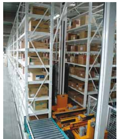
Automated storage for original packs (with rotary racks)
