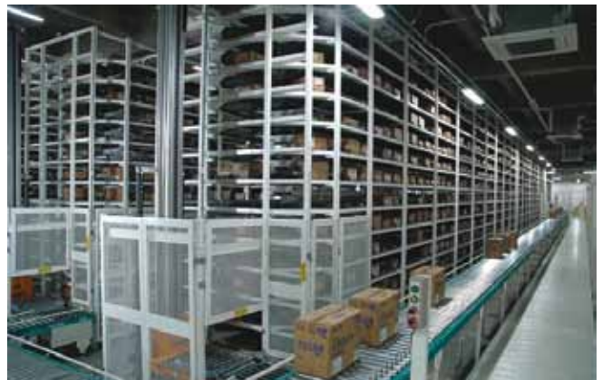
Automated storage for original packs (with rotary racks)
