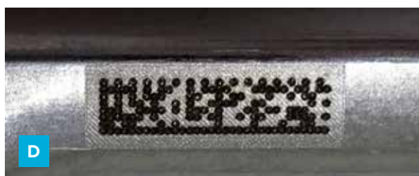
The GS1 DataMatrix barcode laser engraved on a steel instrument: 2.5 mm (C) and 1.3 X 5.0 mm (D).
