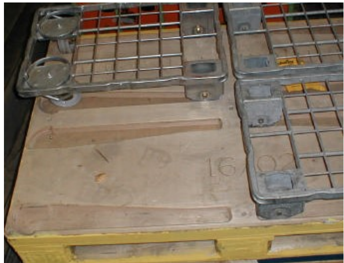
Figure 25: adapter pallets of Fa. Gebhardt and Fa. Container Centralen
