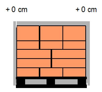
There must not be a pallet goods-shifting, because otherwise the pallet cannot be placed onto the conveyor.
