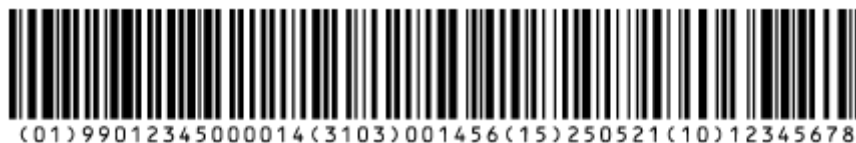
Illustration: GS1-128 Barcode for variable weight item incl. net weight
