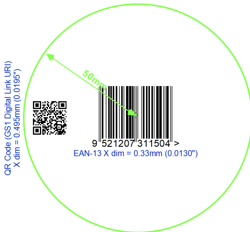
Figure 6-4 2D barcode placement in relation to the linear barcode
