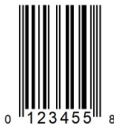
Figure 5-14 UPC-E barcode (encoding 012345000058 by zero-suppression)
