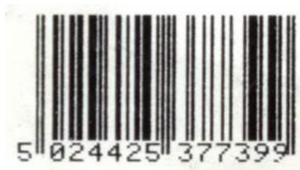
Figure 5-71 Symbol with edge determination problem
