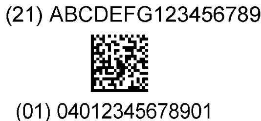
Figure 2-17 Example of GS1 DataMatrix symbol encoded with GTIN and serial number AI (21)
