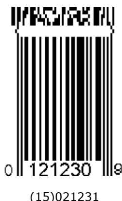
Figure 7-14 Example of mixed GS1 symbologies (GTIN encoded in UPC-E, Best before date in Composite)
