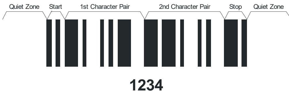
Figure 5-31 ITF-14 symbol inclusive of Quiet Zones
