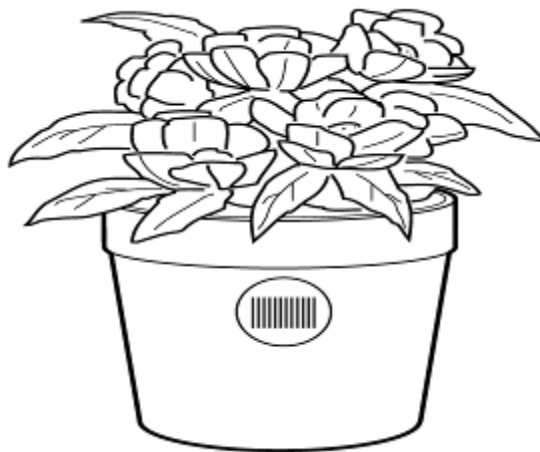
Figure 6-11 Barcode placement with a spot label
