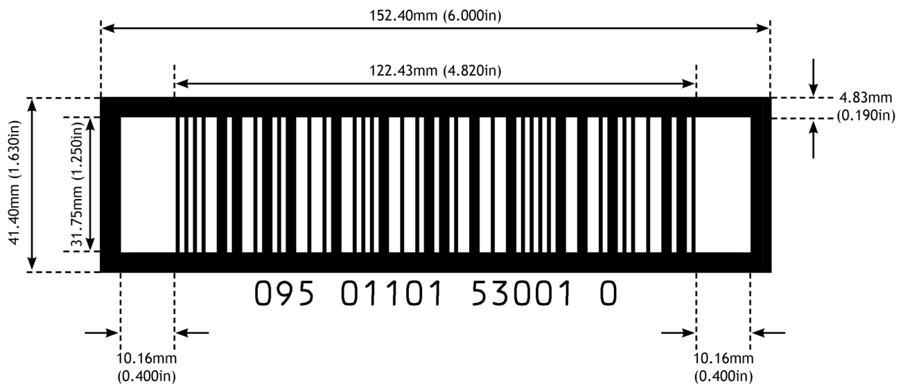
Figure 5-33 ITF-14 symbol: Main dimensions at X-dimension 1.016 mm (0.0400 in.)
